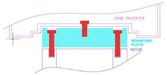
As a first step, the mounting plate must be fixed on the motors terminal box, using original gasket. After the mounting plate is in place, the inverter can be fixed on the plate, using adequate screws and gasket, coming with the plate kit. Specific holes in the capacitor board allow access to the screws inside the inverter.
