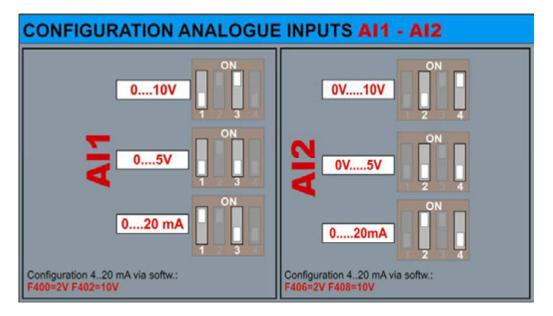
Input impedance for voltage control: 10 kOhm Burden resistor for current loop: 250 Ohm
